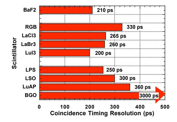
All New Scintillators are Capable of Time-of-Flight
