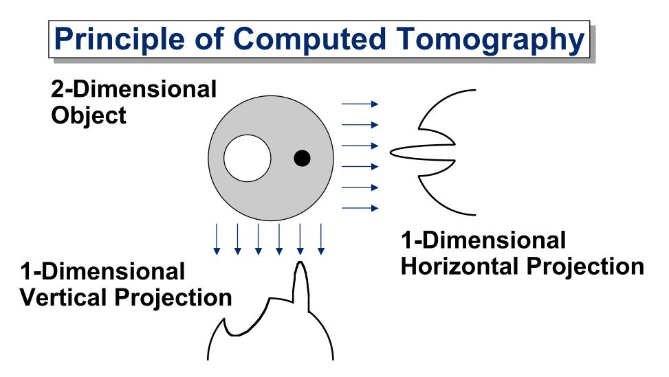
By measuring all 1-dimensional projections of a 2-dimensional object, you can reconstruct the object
