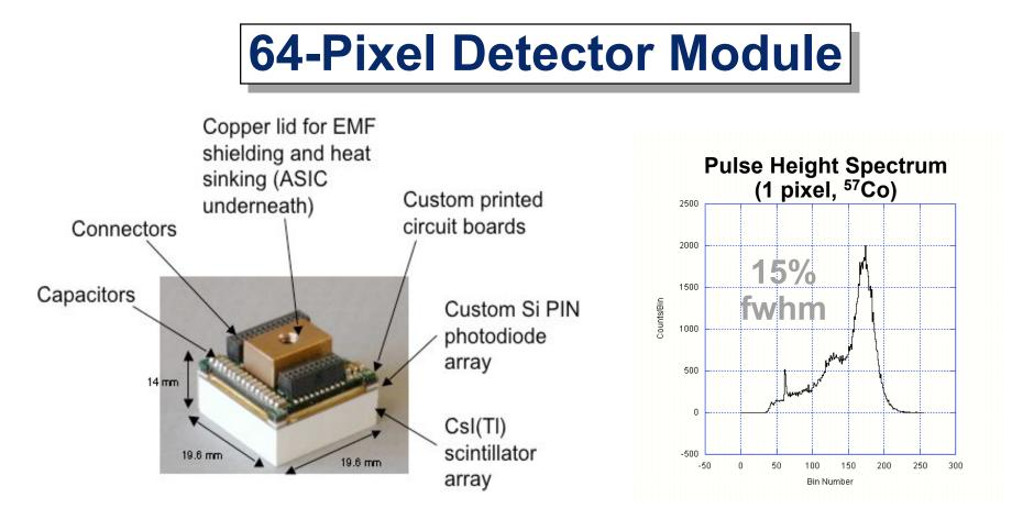
Photodiode Array Developed by LBNL Microsystems Lab
