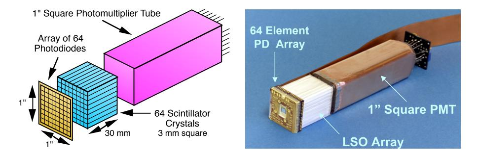
PMT Provides Timing Pulse
